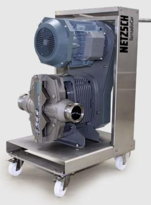
Mobile pumps: For applications in the food and beverage industry, where mobilty and flexibility are required. Mobile units are designed to meet customer specification and requirement.
